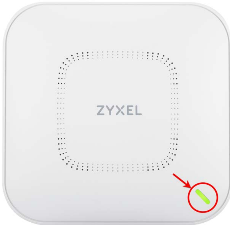
Figure 16 WAC500, NWA1123Acv3, NWA110AX, NWA210AX, WAX510D, WAX610D and WAX650S LED
